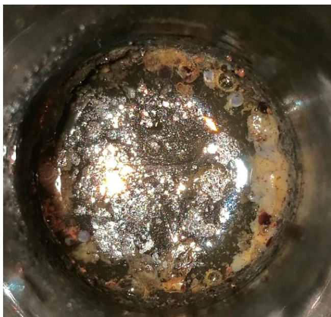
Figure 2: Picture of the typical product behavior after HTL of RMS in the presence of CoMo/Al 2 O 3 once the reactor was opened.
