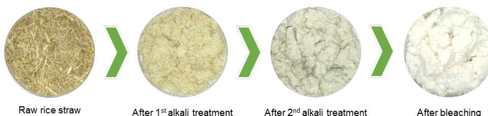
Figure 1: Rice straw appearance after chemical treatments
