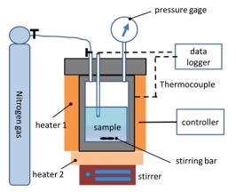
Figure 2: Hot-compressed water treatment apparatus.
