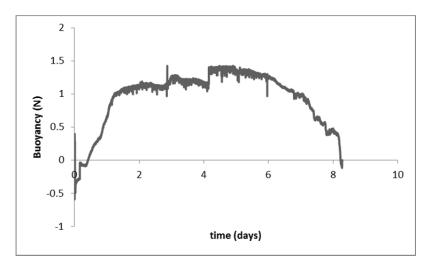
Figure 3: Recorded buoyancy of the pomace cap during the alcoholic fermentation.
