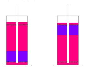
Figure 1: Representation of the two-plate measurement system. In the picture the juice is represented in red, while the cap in purple. The left picture shows the case of sank berries (negative force values), while the right picture the case of floating pomace cap (positive force values).
