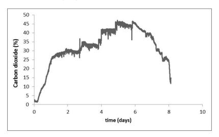
Figure 4: Calculated volume (%) occupied by the carbon dioxide in the pomace cap.
