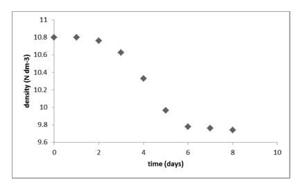
Figure 2: Measured density during the alcoholic fermentation as a function of time.
