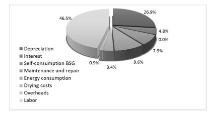
Figure 1: Percentage breakdown of annual operating costs of the small plant of pellets production in relation to 1,600 h  $y^{-1}$  of usage
