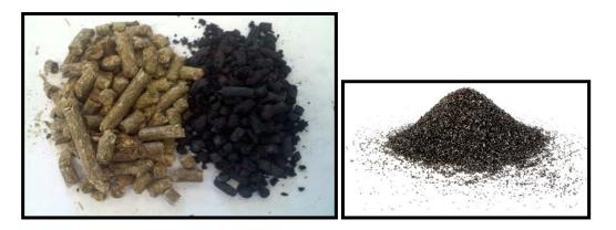
Figure 4: Biochar production from BSG-pellets and bulk BSG
