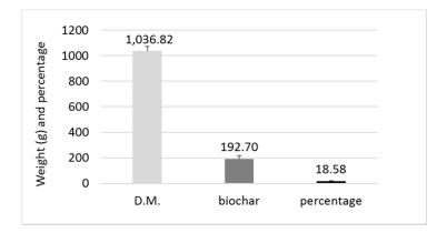
Figure 3: Biochar production from BSG (mean values and standard deviation)
