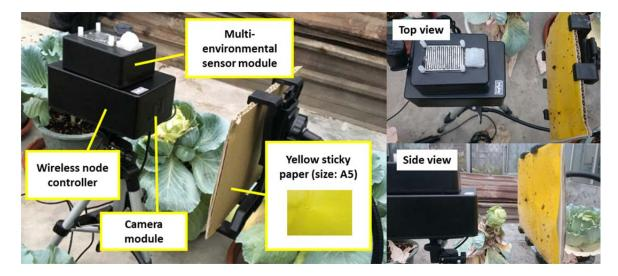
Figure 1: Wireless imaging and sensor node (top view and side view) with part labels
