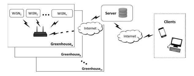
Figure 2: Insect pest monitoring system over-all system structure
