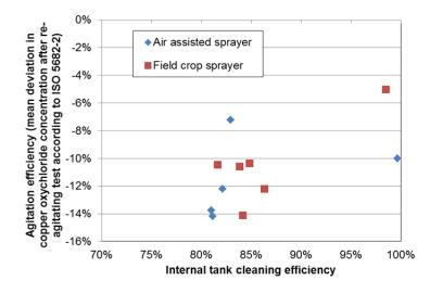
Figure 7: Comparison between efficiency of internal tank cleaning systems measured according to ISO 22368-3 and efficiency of the tank agitation system measured according to ISO 5682-2 in some ENTAM certified sprayers.
