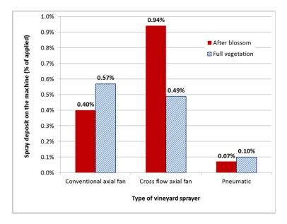
Figure 3: Spray deposits on the external parts of the sprayers measured in vineyards using different machines and operating at two growth vine stages. Experiments were made by DiSAFA applying a test solution of water and yellow dye E102 Tartrazine.
