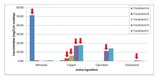
Figure 5: Concentrations of a.i. detected in the washings from external cleaning of a vineyard pneumatic sprayer after each treatment. The red arrows indicate treatments where the specific a.i. was applied (DiSAFA tests 2016).
