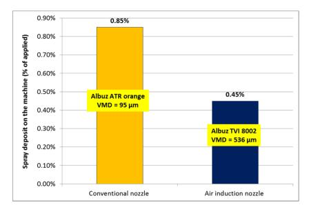
Figure 4: Spray deposits on the external parts of the sprayers measured in vineyards using different nozzle types and droplet sizes, operating at 1.0 MPa pressure and using a cross flow axial fan. Experiments were made by DiSAFA applying a test solution of water and yellow dye E102 Tartrazine.
