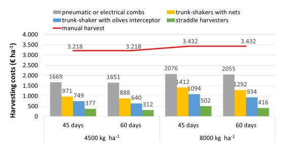
Figure 2: Estimation of olive harvesting costs per hectare for the different mechanization levels for different olive production and harvest period.
