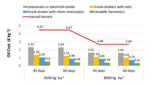
Figure 3: Estimation of olive harvesting costs per unit of oil ( $\in kg^{-1}$ ) for the different mechanization levels in relation to the different olive productions and harvesting period.
