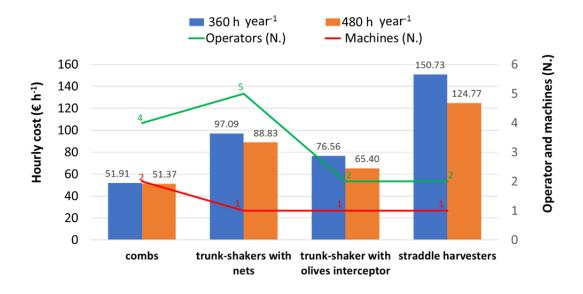
Figure 1: Operating costs of olive harvesting for the different levels of mechanization and labor employed.
