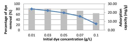
Figure 5: Effect of dye concentration on adsorption of Methyl Orange dye (contact time = 240 min, adsorbent dosage = 0.1 g/50 mL, pH = 7, temperature = 30 gC)
