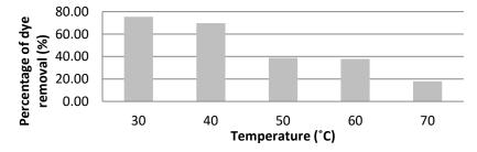
Figure 6: Effect of temperature on adsorption of Methyl Orange dye (contact time = 240 min, adsorbent dosage = 0.1 g/50 mL, pH = 7, dye concentration= 0.05 g/L)
