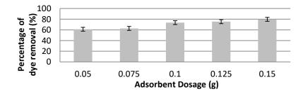
Figure 4: Effect of adsorbent dosage on adsorption of Methyl Orange dye (contact time = 240 min, pH = 7, dye concentration = 0.05 g/L, temperature = 30 °C)
