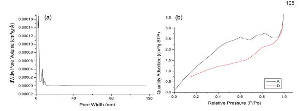
Figure 1: (a) Adsorption and desorption isotherm of nitrogen on PEI modified sugarcane bagasse, (b) Pore size distribution of PEI modified sugarcane bagasse
