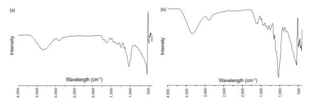
Figure 2: FTIR analysis of (a) raw SB and (b) PEI modified SB
