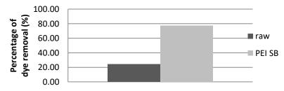
Figure 8: Comparative study between Raw SB and PEI modified SB at optimum condition (contact time = 240 min, adsorbent dosage = 0.1 g/50 mL, dye concentration = 0.05 g/L, pH = 7, temperature = 30 °C)
