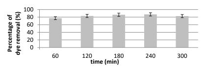
Figure 3: Effect of contact time on adsorption of Methyl Orange dye (adsorbent dosage = 0.1 g/ 50 mL, pH = 7, dye concentration= 0.05 g/L, temperature= 30 °C)
