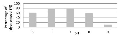
Figure 7: Effect of pH on adsorption of Methyl Orange dye (contact time= 240 min, adsorbent dosage = 0.1 g/ 50 mL, dye concentration = 0.05 g/L, temperature = 30 °C)
