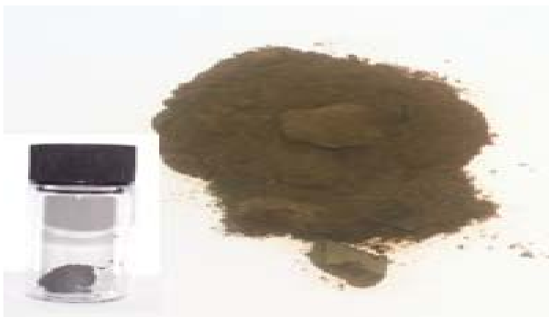
Figure 3: Digital photograph of graphene oxide powder
