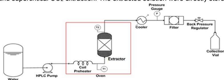
Figure 1: Schematic diagram of subcritical water extraction apparatus
