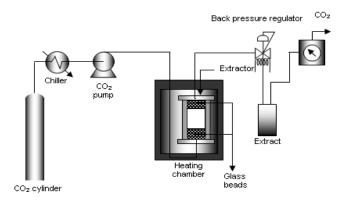
Figure 2: Schematic diagram of supercritical CO2 extraction apparatus
