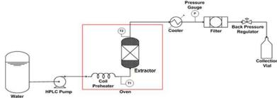
Figure 1: Schematic diagram of subcritical water extraction apparatus
