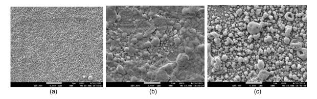
Figure 3: FESEM images of surface of (a) UF PES (20,000× magnification), (b) 4 % TEOA (20,000× magnification) and (c) 8 % TEOA (20,000× magnification)
