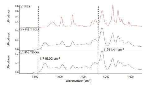
Figure 2: ATR-FTIR spectra of TFC membrane
