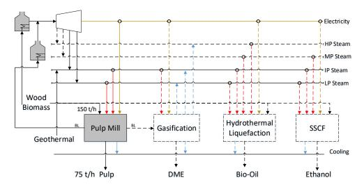
Figure 4: Optimal network showing Kraft pulp as the most profitable processing route.
