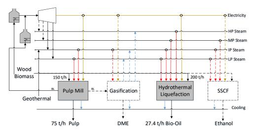
Figure 5: Optimal network with + 5 % increment in biorefinery product prices.
