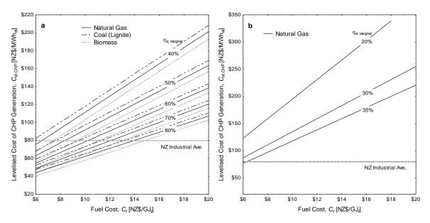
Figure 2: Levelised cost of power generation using back pressure steam turbines (a) and gas turbine (b) at different efficiency of electricity generation. A carbon price of NZ\$18/t<sub>CO2-eq</sub> is included.
