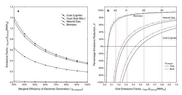
Figure 1: Emissions factor for CHP power generation (a) and percentage emissions reduction per unit of power generated using CHP (b).
