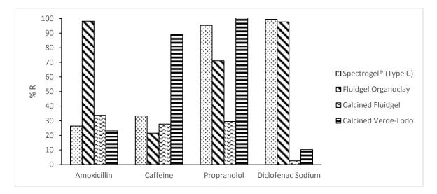
Figure 1: Percentage removal of amoxicillin, caffeine, propranolol, and diclofenac sodium by different clays.
