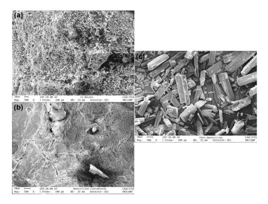
Figure 2: SEM micrographs (500x magnitude) of Fluidgel organoclay (a) prior adsorption, (b) after amoxicillin adsorption, (c) pure amoxicillin.
