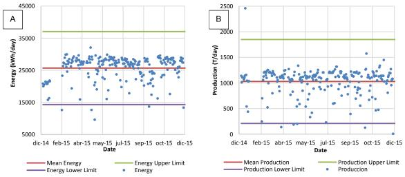
Figure 2. Boundary control charts a) Energy Consumption, b) Equivalent production of fertilizers.
