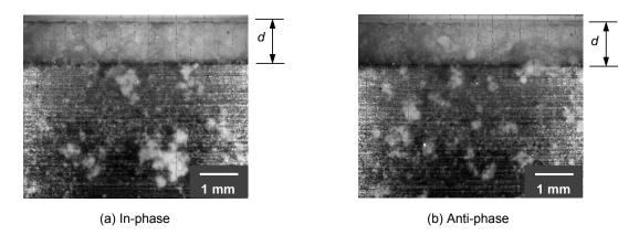
Figure 6: Photographs of powder discharge (SiO<sub>2</sub>, particle diameter  $D_p = 12$  nm, gap distance d = 1.2 mm, vibration amplitude  $A = 20 \mu$ m).
