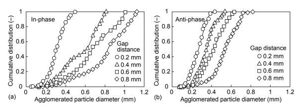
Figure 4: Mass-based agglomerated particle size distribution ( $D_p = 10 \ \mu m$  (Al<sub>2</sub>O<sub>3</sub>), A = 20  $\mu m$ , Tube Inner diameter, I.D.: 18 mm).
