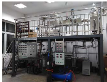
Figure 2: The flow chart and apparatus of two-stage coal dust removal system
