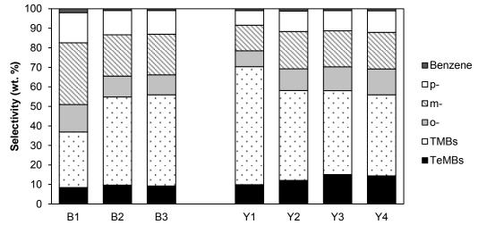
Figure 4: Product selectivity for all tested catalysts at time = 50 hours, T = 400 °C, P = 1.0 Mpa,  $H_2/HC = 4$ , and WHSV = 5  $h^{-1}$
