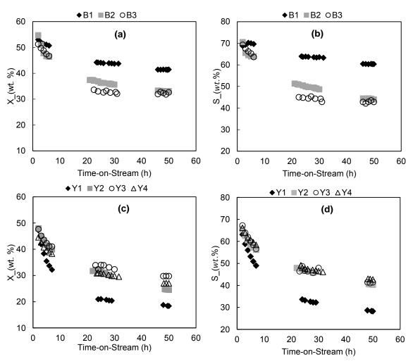
Figure 2: Catalytic conversion (a & c) and selectivity (b & d),  $T = 400 \degree C$ , P = 1.0 Mpa,  $H_2/HC = 4$ , and  $WHSV = 5 h^{-1}$
