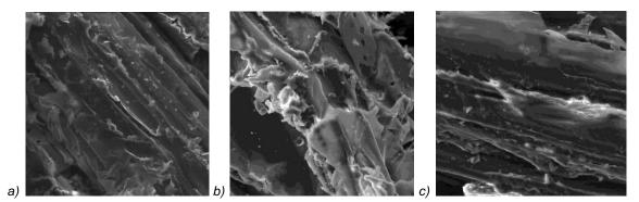
Figure 2: SEM micrographs of: (a) original; (b) ultrasonic treated; (c) NaOH treated hemp hurds samples (4000 times of magnification)
