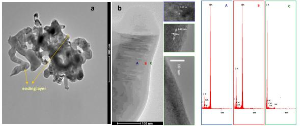
Figure 1: TEM image of  $G/SiO_2/SiC$  (a). Representative TEM images of the prepared nanofilaments of  $G/SiO_2/SiC$  composite. High resolution TEM images of coaxial nanofilaments, displaying single crystalline 3C-SiC core, SiO<sub>2</sub> intermediate layer and outer graphitic carbon sheaths. Energy dispersion spectra taken from different zones of the nanofilaments as marked in Figure 1b with A, B and C.
