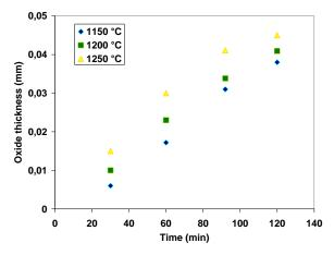
Figure 3: Oxide thickness as a function of time and temperature during tests performed in the same operating condition of the C/SiO<sub>2</sub>/SiC synthesis but temperature.
