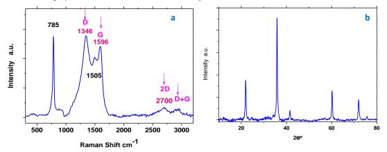
Figure 2: Raman spectrum of G/SiO<sub>2</sub>/SiC (a) and X-ray diffraction spectrum of G/SiO<sub>2</sub>/SiC (b).
