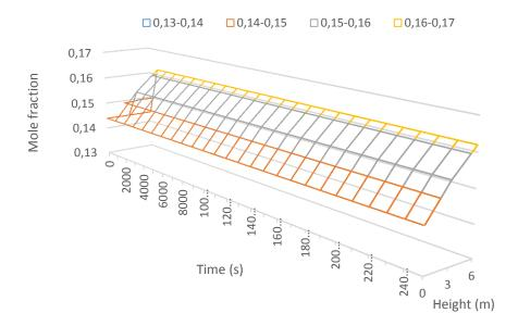
Figure 2: Concentration of carbon dioxide from dense bed - simulation
