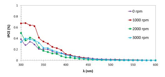
Figure 4: IPCE measurements for the samples anodized at 0, 1000, 2000 and 3000 rpm and annealed at a heating rate of 15 °C·min<sup>-1</sup>.
