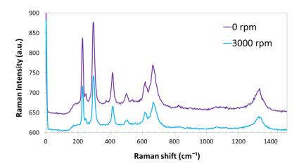
Figure 3: Raman spectra of the nanostructures anodized at 0 and 3,000 rpm
