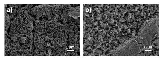
Figure 2: Field Emission Scanning Electron Microscopy images for the nanostructures synthesized at 0 rpm (a) and 3,000 rpm (b).
