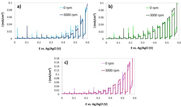
Figure 1: Photocurrent density versus potential measurements for the samples anodized at 0 and 3,000 rpm and annealed at a heating rate of 2 (a), 5 (b) and 15 °C·min<sup>-1</sup>(c).
