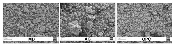
Figure 1: Scanning electron micrographs of samples of: Maltodextrin (MD); Arabic Gum (AG) and Proanthocyanidins (OPC).
