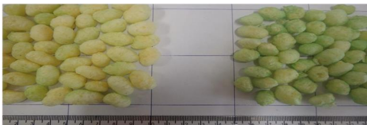
Figure 1 – Preliminary coating test result. On the left, 100 g of the maize starch solution for each kilogram of snacks and on the right, 320 g of the maize starch solution for each kilogram of snack.
