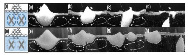
Figure 7: Direction of the impellers rotating (i) centre-down and (ii) centre-up. Images of two different islands detached from the interface. From (a) to (d) island experienced centre-down rotation and from (e) to (h) island experienced centre-up rotation ( $V_f$ =0.15,  $d_p$ =0.75-1.00 mm)
