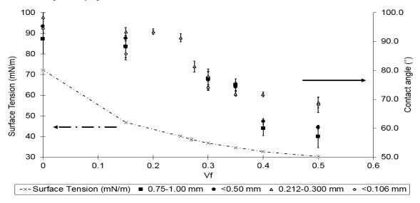
Figure 3: Contact angle of silanised glass beads of different diameter,  $d_p$  as a function of the liquid ethanol volume fraction,  $V_f$ . The crosses refer to the surface tension as a function of  $V_f$ .
