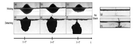
Figure 5: Images of islands at  $V_F=0.15$ , (a)-(c) experienced wicking (for  $d_p=0.75$ -1.00 mm), (d)-(f) experienced detaching from the interface (for  $d_p=0.212$ -0.300 mm). Images of the system that can only support rafts instead of islands at  $V_F=0.40$ .  $V_F=0.212$ -0.300 mm (g) and  $V_F=0.212$ -0.300 mm (h).
