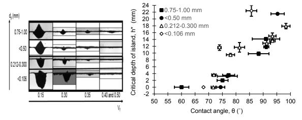
Figure 4: Critical island depth,  $h^{\dagger}$ , formed by silanised glass beads of different  $d_p$  at different  $V_f$  (left). Effect of the bead contact angle and particle size on the critical island depth,  $h^*$  (right).
