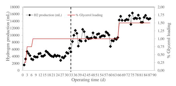
Figure 3: Hydrogen production and glycerol loading during fermentation in 20 L semi-continuous bioreactor.
