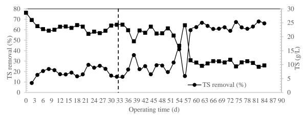
Figure 4: The efficiency of TS removal during fermentation in 20 L semi-continuous bioreactor.
