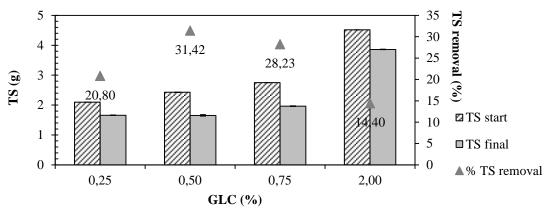
Figure 1: The efficiency of TS removal at the varying glycerol loading of 0.25-2% GLC.
