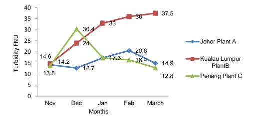
Figure 3: Variation of turbidity of the effluent wastewater treatment
