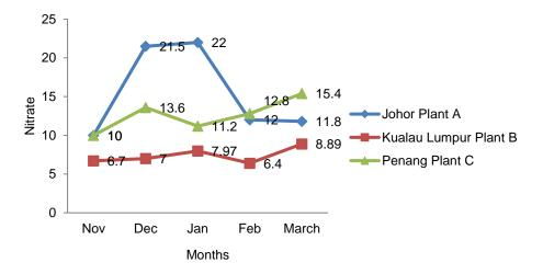
Figure 5: Variation of Nitrate for the effluent wastewater treatment
