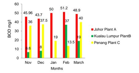
Figure1: Variation of BOD in the effluent domestic wastewater plants
