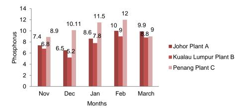
Figure 6: Variation of Phosphorus for the effluent wastewater treatment
