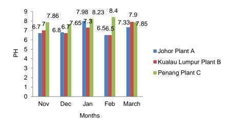
Figure 4: Variation of PH in the effluent STP plants
