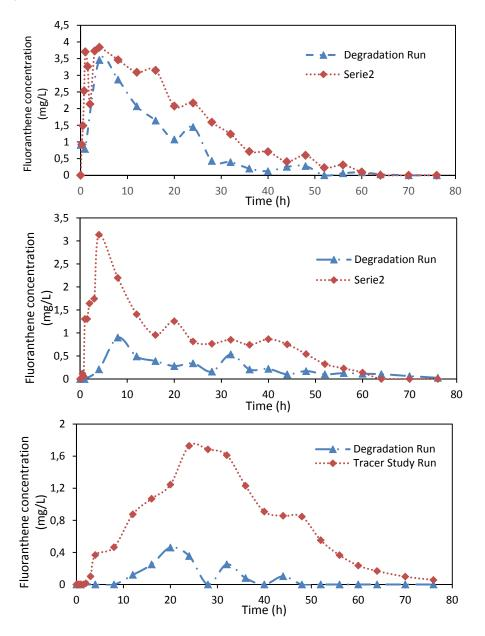
Figure 4: Effluent fluoranthene concentration 'blue' from (a) PAH biodegradation zone 2A, (b) biodegradation zone 2B, and (c) final removal of PAH residual in the biofilm reactor with tracer concentration (red) respectively
