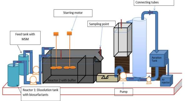
Figure 1: Diagram showing the layout of the CSTR-Biofilm reactor connected in series with dual feed for growth medium and PAH dissolution chamber
