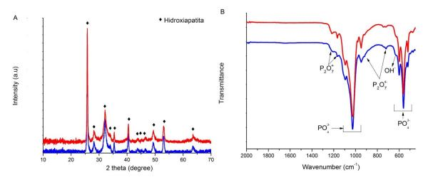
Figure 2: (A) XRD patterns of coating on Ti6Al4V (blue line) HAP (red line) HAP/CNT and (B) FTIR spectra of coating on Ti6Al4V (blue line) HAP (red line) HAP/CNT.
