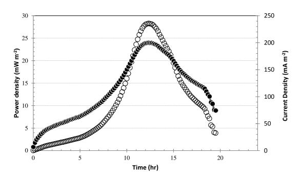
Figure 2: Power (O) and Current density (•) from tannery wastewater in MFC
