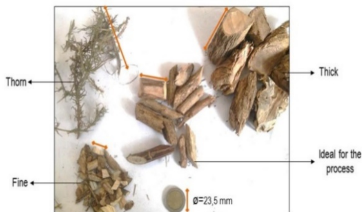
Figure 2. After granulometric reduction and screening
