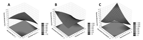
Figure 3: Response surface plots and contour plots for maximum removal efficiency for the 28 experimental runs carried out under conditions established by CCRD; removal efficiency as function of (A) oily water flow and microbubble flow; (B) oily water flow and biosurfactant concentration; (C) biosurfactant flow and biosurfactant concentration.
