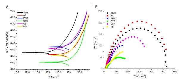
Figure 3. Electrochemical response of the surface-modified steel in physiological solution. (A) linear sweep voltammetry, (B) Nyquist diagram obtained from electrochemical impedance spectroscopy evaluation.
