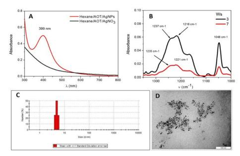
Figure 1. Properties of Ag NPs in hexane/AOT/water. (A) Absorption spectra at Ws=7. Empty RMs were used as blank. (B) Infrared absorption of asymmetric and symetric S=O stretching at Ws=3 and 7. (C) DLS histogram and (D) TEM image of Ag NPs in hexane/AOT Ws=7.
