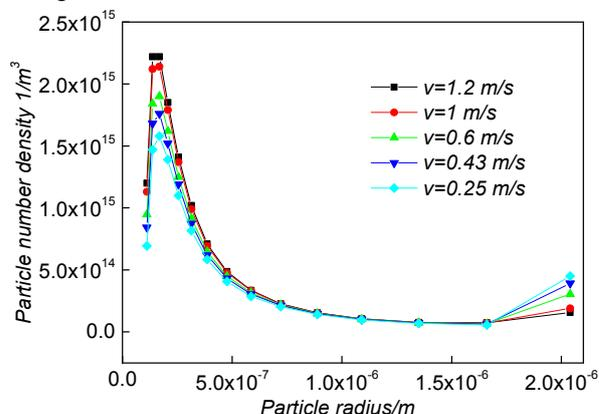
Figure 5: Flow gas velocity effect on fine particles enlargement
