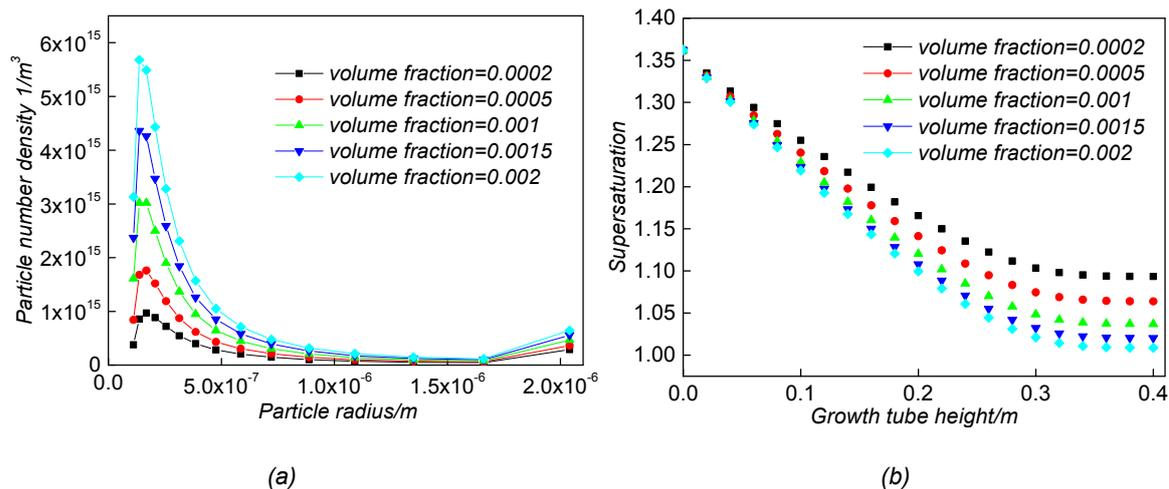
Figure 6: (a) Volume fraction effect on fine particles enlargement (b) Supersaturation distribution in the growth tube
