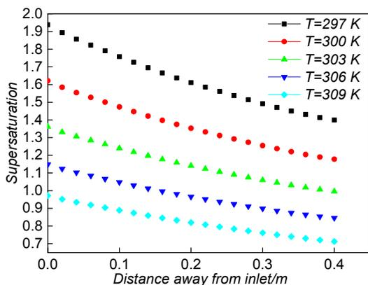
Figure 2: The profile of supersaturation in the axis of growth tube
