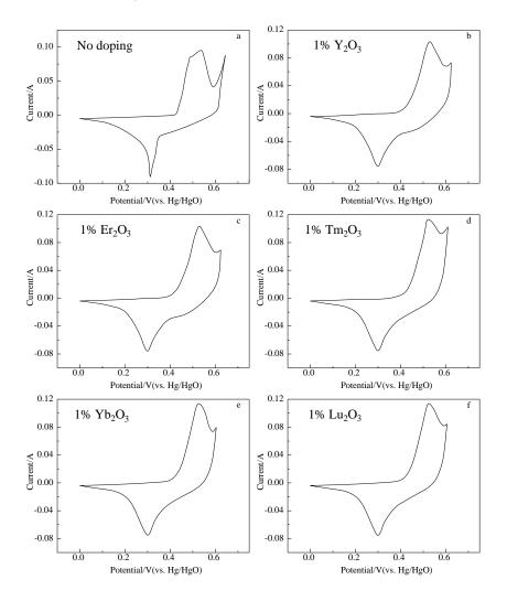
Figure 4: Curve of volt-ampere characteristics of different types of Ni-MH Batteries at room temp.
