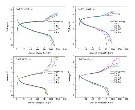
Figure 1: Charge-discharge curve of Ni-MH Batterie with REOs
