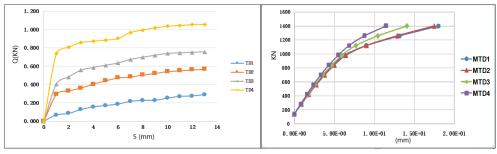
(a) The load-displacement curve of TD1 $\sim$ TD4 (b)The load-displacement curve of MTD1 $\sim$ MTD4
