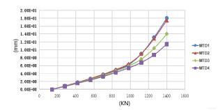
Figure 10: The L-D curve of a fixed point on the pile top under different vertical loads
