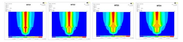
Figure 9: The Y-direction soil displacement of model piles with different suspension plate diameters
