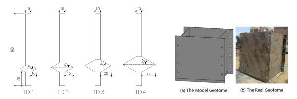
Figure 1: Design charts of the CEP pile with different diameters Figure 2: The geotome
