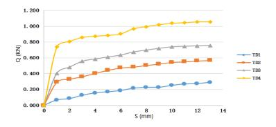
Figure 8: The contrastive S-Q curves of Model piles TD1, TD2, TD3, TD4
