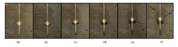
Figure 3: The whole process of soil destruction of Pile TD2
