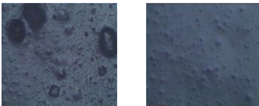
Figure 1: Optical microscope photographs (100X) of API filter-cake: bentonite(left) and SLRP(right)
