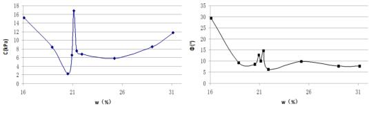
Figure 3: C ~  $\omega$  curve
