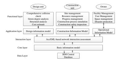
Figure 4: Logical structure of green building materials supply chain information flow model based on BIM
