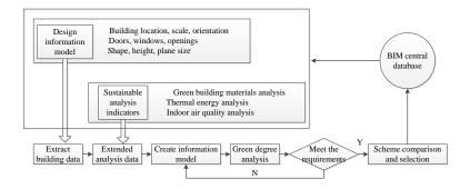
Figure 5: Information flow for green building materials analysis based on BIM
