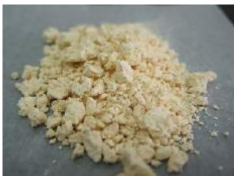
Figure 6: Microcapsules of phase change materials with eighteen alkanes as core materials
