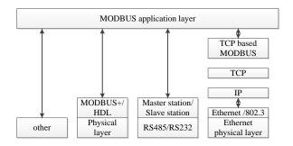
Figure 1: Modbus communication stack
