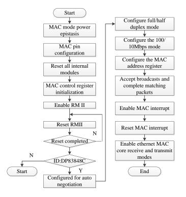
Figure 4: Ethernet software initialization program
