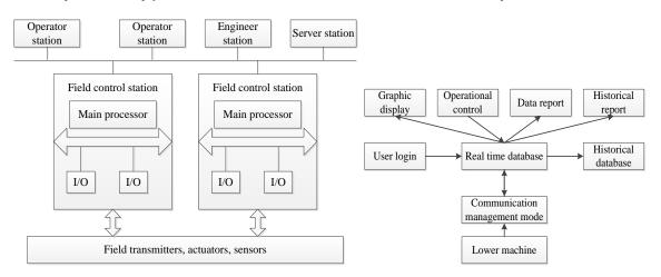
Figure 6: Typical distributed control system architecture Figure 7: Real-time database transaction scheduling
