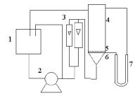
1. Sink; 2. Magnetic pump; 3. Rotameter; 4. Fluidized bed; 5. Distribution board; 6. Predistributor; 7. U-tube differential pressure meter
