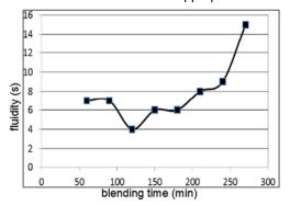
Figure 6: The Relational Graph of the Large Cooker Car's Fluidity and Blending Time
