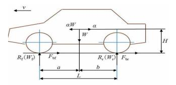
Figure 1: The force of the car when braking on the horizontal road
