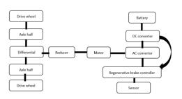
Figure 2: Central motor type regenerative braking system
