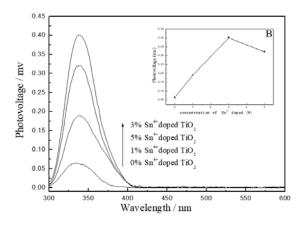
Figure 7: Surface photovoltage comparison of TiO<sub>2</sub> nanoparticles doped with different tin contents (molar concentration) at an annealing temperature of 400°C Figure B shows the change curve of surface photovoltage with different tin contents at 400°C
