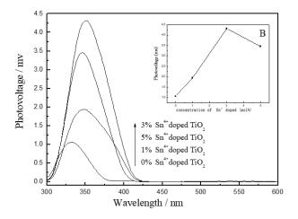
Figure 8: Surface photovoltage comparison of  $TiO_2$  nanoparticles doped with different tin contents (molar concentration) at an annealing temperature of 600°C Figure B shows the change curve of surface photovoltage with different tin contents at 600°C
