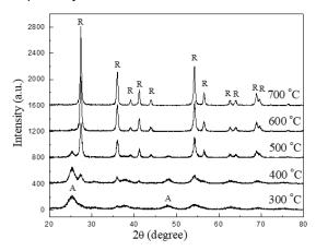
Figure 1: XRD pattern of pure and 5 mol% tin-doped TiO<sub>2</sub> nanoparticles
