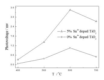
Figure 6: Comparison of surface photovoltage intensity of pure TiO<sub>2</sub> nano-particles and TiO<sub>2</sub> nano-particles doped with different tin contents at different annealing temperatures
