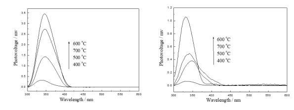
Figure 4: SPS of pure TiO2 nanoparticles at different annealing temperatures
