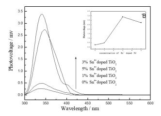
Figure 9: Surface photovoltage comparison of TiO<sub>2</sub> nanoparticles doped with different tin contents (molar concentration) at an annealing temperature of 700°C Figure B shows the change curve of surface photovoltage with different tin contents at 700°C
