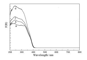
Figure 3: The function curve of wavelength and F(R) of pure TiO<sub>2</sub> nanoparticles (wherein, a denotes the case without doping, b with content of 1mol% tin, c with content of 3mol% tin, and d with content of 5mol%tin)
