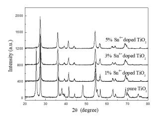
Figure 2: XRD pattern of pure  $TiO_2$  nanoparticles and  $TiO_2$  nanoparticles doped with different contents of tin at an annealing temperature of 600 °C
