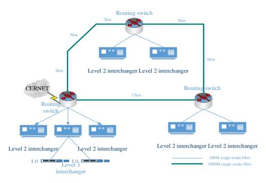
Figure 1: Chemical enterprise network backbone topology
