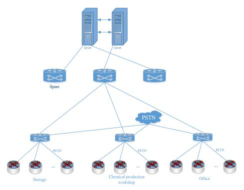
Figure 2: Hierarchical design network topology
