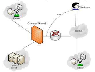
Figure 3: Chemical company network security diagram.
