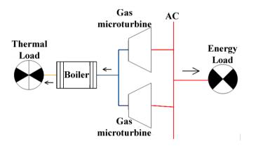
Figure 1. CHP system scheme
