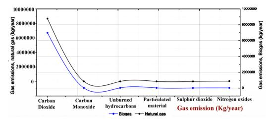
Figure 7. Gas emission comparison for Biogas and Natural gas
