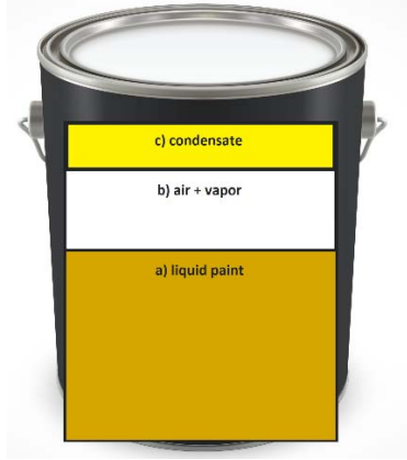
Figure 1. Sketch of the system under consideration: a) liquid paint phase; b) air and vapor phase; c) condensed phase.
